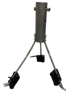
Figure 18: Custom-made tripod in Aluminium for the MinidotPE. Made in DTU-skylab
