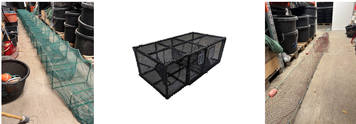
Figure 15: Gear used for fishing. Left: Netted lobster trap. Middle: Rigid lobster trap. Right: Eel fyke
